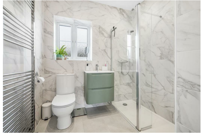
PVC double glazed window to side. Skimmed ceiling. Recessed spot lights. Extractor fan. Vinyl tiled flooring. Full height wall tiling. Chrome heated towel rail. Fitted with a three piece suite comprising walk in shower enclosure with Aqualisa shower. Close coupled toilet with push button flush. Pedestal wash hand basin set in vanity unit with built in storage.
